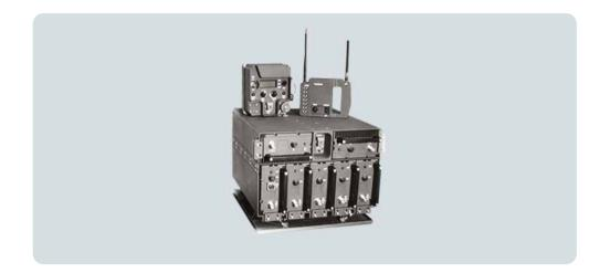
The family of devices ELT/334 is used for radio activation systems jamming of explosive devices called RC-IED (Remote Controlled Improvised Explosive Devices), operating in the VHF/UHF band. The system generates a noise signal, which prevents the activation signal, to arrive intact at the receiver and actuate the explosive device. It is available in man-portable and on-vehicle configurations.
