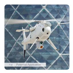
ELT/1001 is a family of Communication ESM systems for installation on UV (Unmanned Vehicle) class II platforms. The product is used in support to land and/or naval military operations by offering electromagnetic passive surveillance for intercepting, classifying, and identifying Communication RF signals over the horizon. It is designed to be employed in light ISR missions performed by small airborne platforms such as Tactical UAVs.
